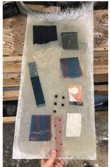
Above: Physical tests and samples exploring the way metal can be sliced and bent to create sharper bends without the need for heavier machinery. Fibre glass tests submerging found fabrics within the third layer of fibreglass.
