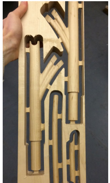
Above: An antler detail milled from multiple types of wood and polyurethane board, joined with a sloping lap joint.
