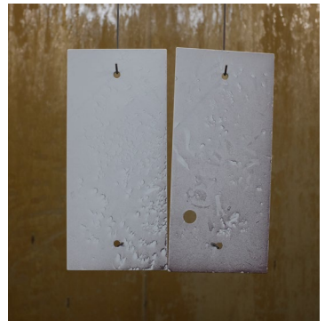
Above: Working closely with manufacturers has allowed for material experimentation here shows a dusting process we have been developing with our powdercoaters. Through a glue residue and manipulation of static we can create shadows of patterns.
